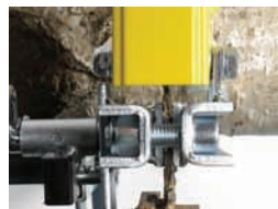
Stable fixation of the saw blade
